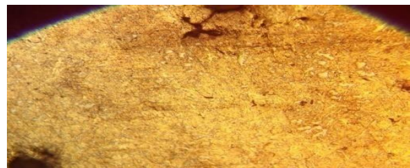
Figure 11b: Micrograph of sample with PKSA at 9%
