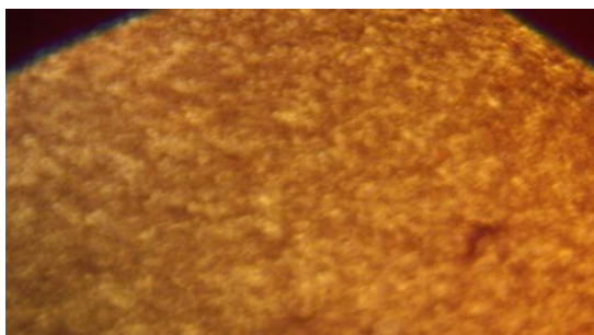
Figure 9a: Micrograph of sample with PKSP at 3%
